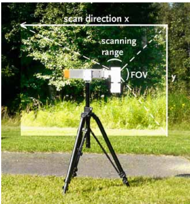
Mirror Scanner mounted on a cased Spectral Camera on top of a standard tripod
