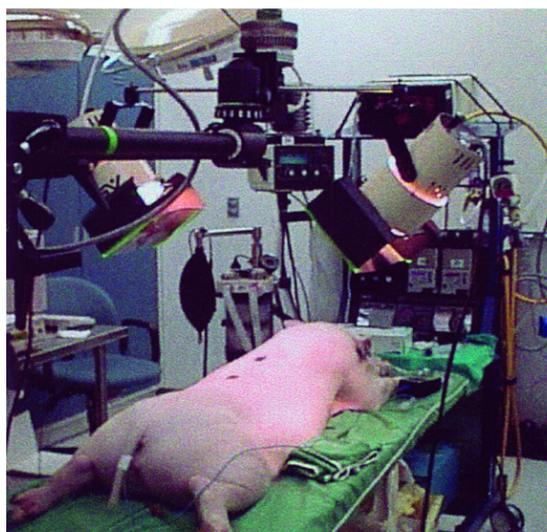
Figure 1 The NIR imaging system provides a rapid and objective assessment of the burn injury.
